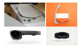
Figure 1. Top: Google Glass viewed in a box [54] and from above [41]. Bottom: Microsoft HoloLens viewed from the side and from the front [56]. Images CC-BY 2.0
